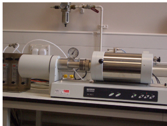
Fig. 2. The dilatometry system used in the study.
